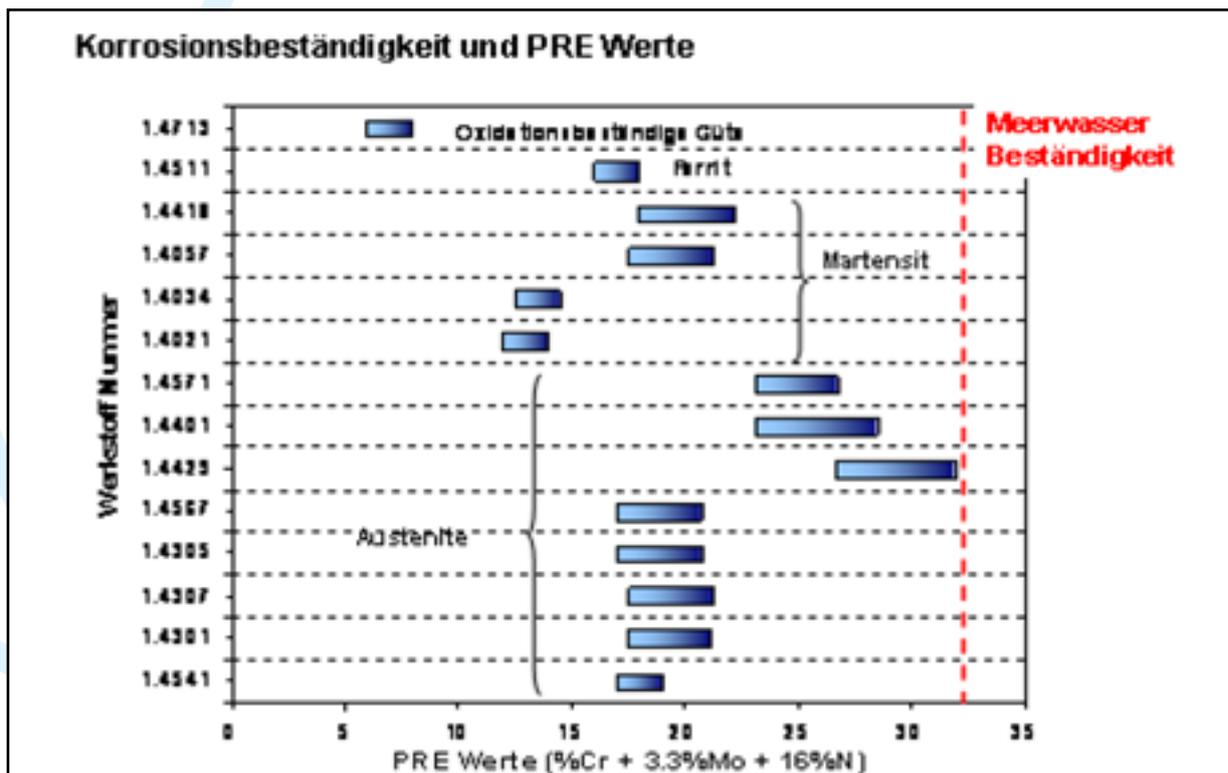
**PRE value:** The value is used to estimate corrosion resistance of a nickel containing alloy against pitting and crevice corrosion. This value is also known under PRE (pitting resistance equivalent).
